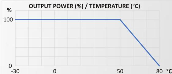
Thus if the charger is forced to operate in an environment above  $+50^{\circ}\text{C}$ , it will simply reduce its output power to the corresponding value in the above chart and continue normal operation.
