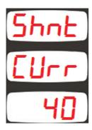
This parameter adjusts the rated value of the current shunt in amperes.
