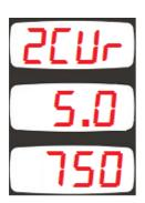
In the second current input sensitivity calibration mode, the first display will show "2CUR". The second screen will display the measured instantaneous current from the input. The third display will display the calibration coefficient (high 4 digits only)
