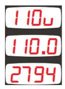
The calibration screen about the 110V voltage input will be seen. The first display will show "110V". The second screen will display the measured instantaneous voltage from the input. The third display will display the calibration coefficient (high 4 digits only)
