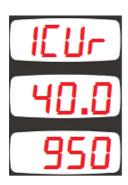
In the first current input sensitivity calibration mode, the first display will show "1CUR". The second screen will display the measured instantaneous current from the input. The third display will display the calibration coefficient (high 4 digits only)
