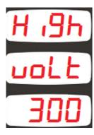
This parameter adjusts the upper limit of the high voltage alarm. If this parameter is set to 300 then high voltage is not monitored and
