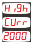
This parameter adjusts the overcurrent limit.
