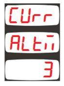
This parameter determines the delay between a high current alarm condition occurs and the alarm given.
