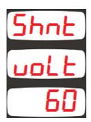
This parameter adjusts the rated voltage of the current shunt in milivolts.
