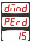
This parameter determines the demand period for voltage, current and power measurements. The average value is calculated during the demand period and at the end of the period new demand values overwrite older values.
