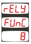
This parameter determines the relay function which dedicates using relay in which alarm(s).
