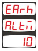
This parameter determines the delay between an earth leakage alarm condition occurs and the alarm given.
