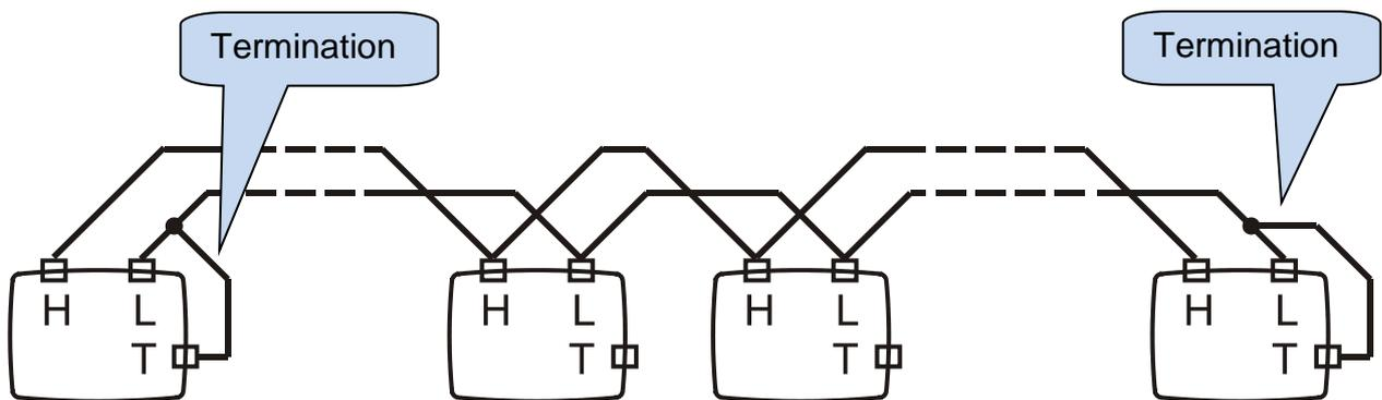
Figure illustrating the Datalink termination from two ends
