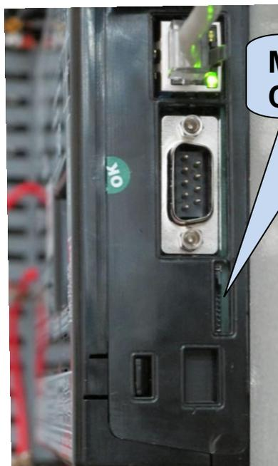
The micro-SD card slot is available in units with COMM option. The slot is of push-in push-out type. When pushed in, the card is firmly held by its connector.
