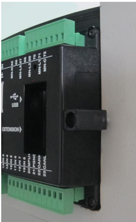
Installation of screw type bracket
